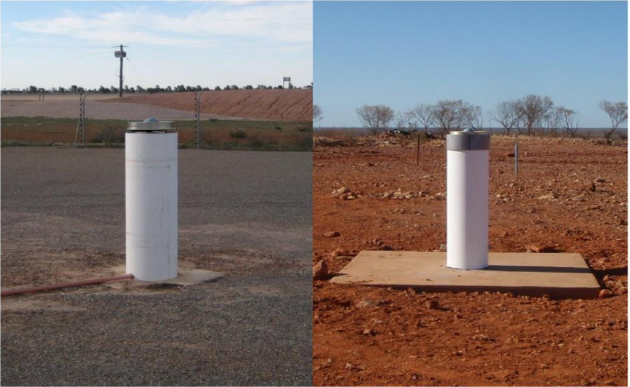
Figure 19 : Sample monumentation of CORS in Australia (Source: ICSM, 2020)
